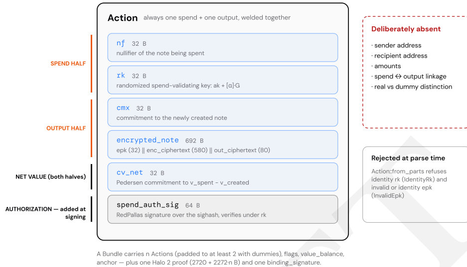
Figure 7: Anatomy of an Action. Action::from_parts rejects an identity rk and an invalid or identity epk at parse time, mirroring consensus rules.
